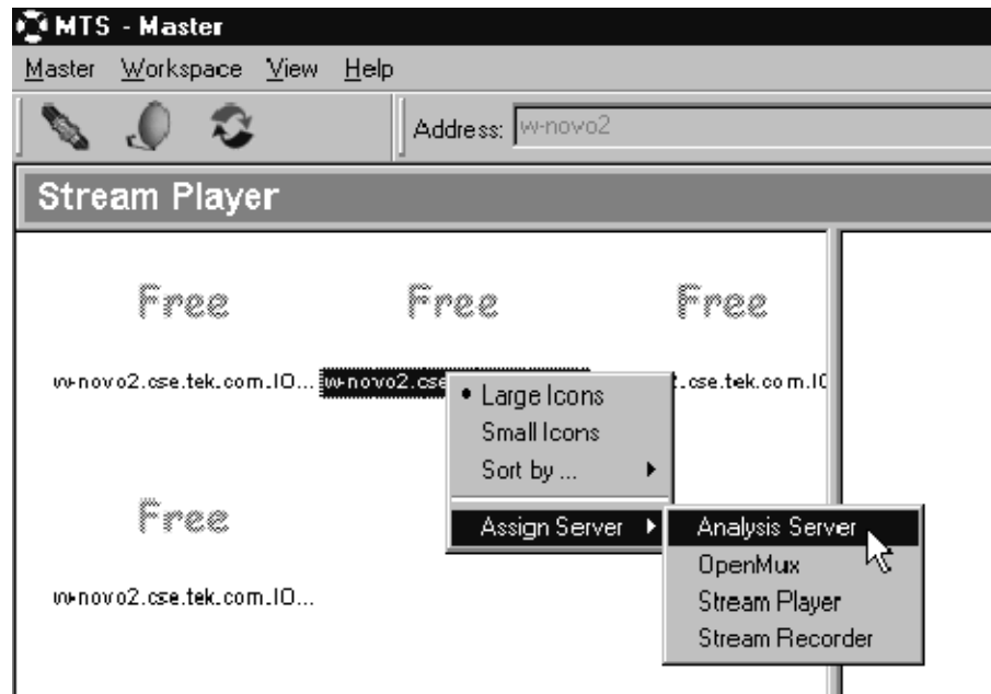
Figure 2-29: Port Manager panel showing Analysis Server selected
